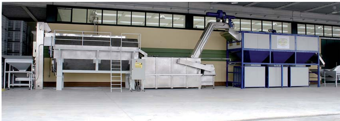
Sterilization line: Endless device for in shell Chestnuts, complete with cooling tank, skimming, dropping and drying for loads up to 1600-5000 kg/hour
