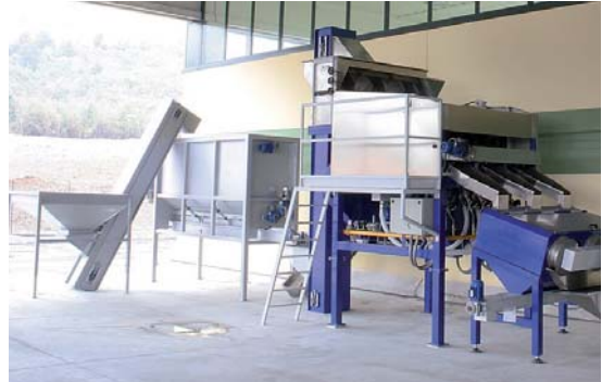
Brulage and steam chestnut peeling line with pre-dryer (8000 kg /h)
