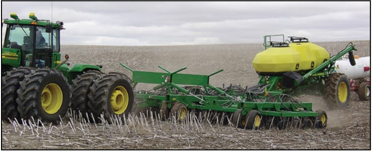
Figure 14. This one-pass seeding operation is seeding directly into wheat stubble. Anhydrous ammonia and seed are banded through special openers. (Roger Ashley, NDSU)
