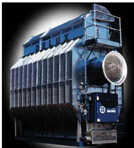
Figure 128. A high-temperature column dryer used for drying sunflower. (Kenneth Hellevang, NDSU)
