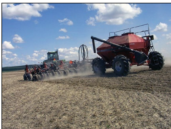
Figure 13. Air-seeder with sweeps used for minimum till sunflower planting. (Roger Ashley, NDSU)
