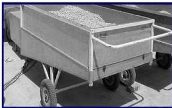
Figure 7. Wagon Bin dryer
