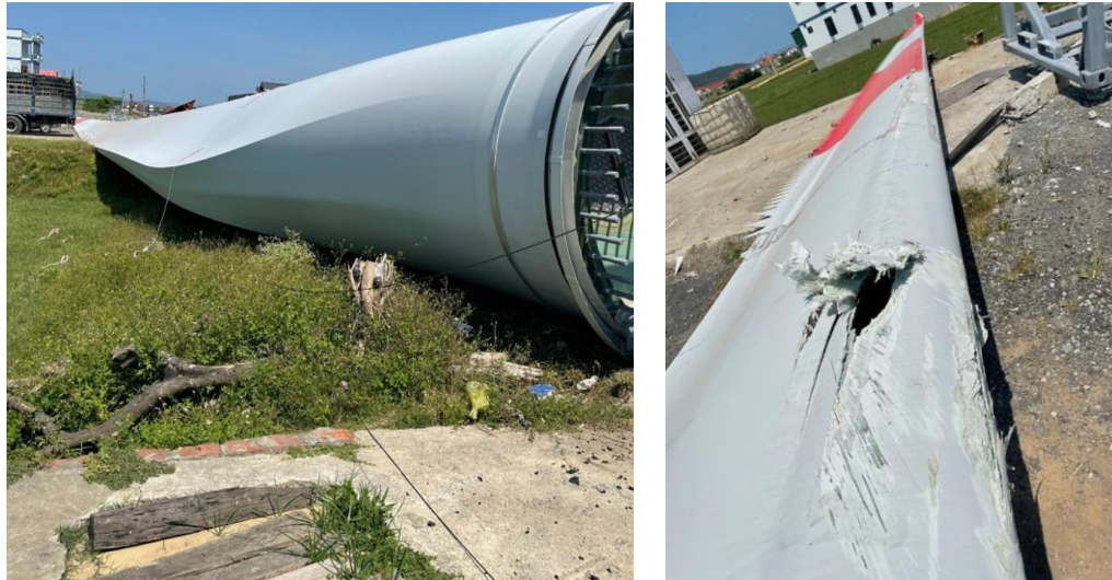
Figure 13.2 Traffic Accident in Quang Binh Province during the Transportation of Wind Turbine Blade (May 2021)
