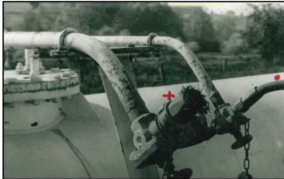
"Station" valves (cross = broken liquid hose, dot = gas hose); valves on the booster side in back of the tanker trailer (2)
