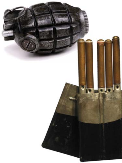
Part of the ANTHROPOID equipment consisted of British Mills hand grenades, model 36M Mk.I, and what are called timing pencils. They were pencil fuses with different delay times.
