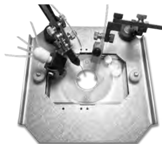
QS-U-R-TT-O Round unheated chamber in Olympus round stage adapter and square Tool tray with StageHands.
