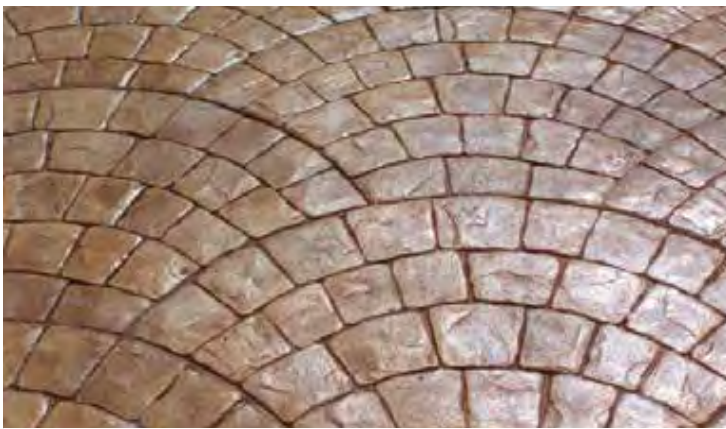
London Cobble Strip, FM-560 S/O 5.75" x 28.625" (14.605 x 72.71 cm) Blue Matching skin/touch-up wheel: Slate/ FM-6510 Joint 1/8"-1/4" wide, 1/4" deep Stone size 5 1/2"-5 3/4" wide, 5 1/4"-8" long
