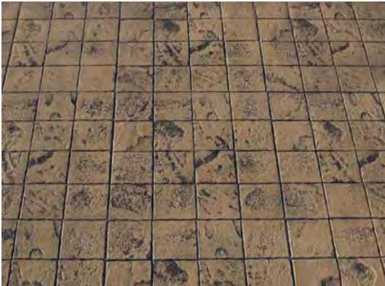
6" x 6" Granite Sets, FM-250 S/O 24" x 24" (60.96 x 60.96 cm) Blue Matching skin/touch-up wheel: Rough Stone/ FM-6510 Joint size \frac{3}{8} "- \frac{1}{2} " wide, \frac{1}{4} " deep Stone size 5 \frac{3}{4} "
