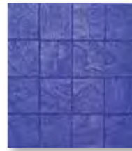
6" x 6" Granite Sets, FM-250 S/O 24" x 24" (60.96 x 60.96 cm) Blue Matching skin/touch-up wheel: Rough Stone/ FM-6510 Joint size \frac{3}{8} "- \frac{1}{2} " wide, \frac{1}{4} " deep Stone size 5 \frac{3}{4} "
