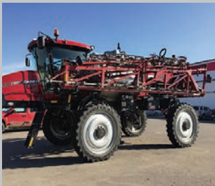
2013 CASE IH PATRIOT 4430 SPRAYER/HIGH CLEARANCE Lux. Surveyor Cab, Active Suspens., 120' Boom, AIM Command, HID Lighting, 320/90R46 & 800/70R38, Front Fill, AccuBoom, Suct. Quick Fill $262,500
