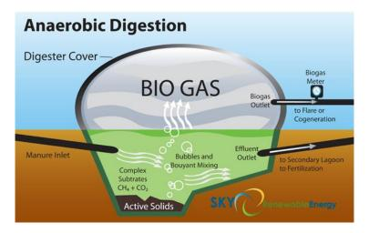
Figure 2: Anaerobic Digestion (Sky Reneable Energy, 2012)
