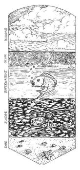
more scum than manure substrates. Scum can also increase with Figure 1: Anaerobic Pond Layers addition of alkaline supplements. It should generally be avoided because
