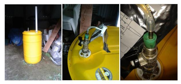
Figure 18: Assembled Prototype Located in Shed Figure 19: Gas Collection after Several Months Figure 20: Photo of Leak around gas outlet
