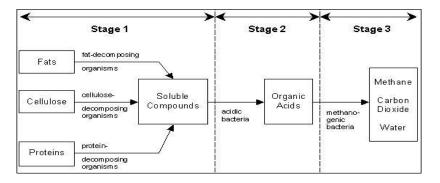
Figure 3: Biological Process for Anaerobic Digestion
