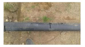
Figure 11: Perforated Pipe from Waikato Dairy Farm
