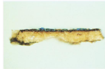
15. Cross-section of a paint sample of the pre-1941 blue sky, showing azurite over a dark grey underpainting and chalk ground.
