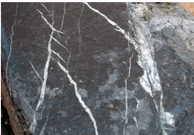
Fig. 6. Boundstone (Namur limestone) with tension joints.
