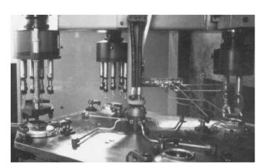
This application shows a multiple-spindle machine with four stations, for machining aluminum covers. An 8-station rotary valve coupling is at the center, with its four unused ports plugged.
