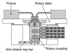
Four-passage rotary coupling with a reaction-bar to prevent stress on hose connections.
