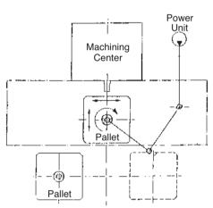
Machining-center pallet changer with continuous fluid feed using Rotary Couplings.
