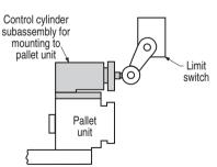
Limit switch mounted on machine table monitors clamping pressure by sensing the extended position of the Control Cylinder's plunger. If system pressure somehow drops below the set level, the plunger would retract.
