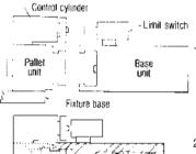
1. Units before coupling (Separated during machining operation).
