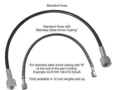
Small-Diameter high-pressure hose perfect for workholding applications. Abrasion and chemical resistant outer cover with seamless nylon inner sleeve reinforced with synthetic yarn. Other lengths and diameters available upon request.
