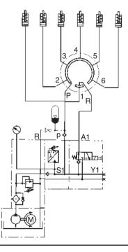
Type 2 Two Stations for Load/Unload **Commonly Controlled**
