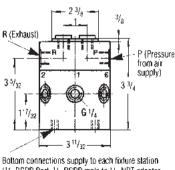
(1/4 BSPP Port, 1/4 BSPP male to 1/4 NPT adapter supplied. Ingestion of pipe dope or lefton tape may cause malfunction or damage to valve)
