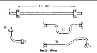
We recommend using tubing clamps as this will increase the life of the installation. Tubing clamps should be less than four feet apart (Figure 1) and bends should be supported also (Figure 2). Use bends as shown in Figures 3 and 4 instead of straight-line connections to prevent stressing the tubing.
