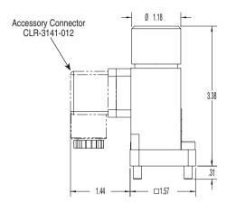
and installations. The switching point can be adjusted to the desired hydraulic pressure via a knurled knob. The knob can be looked in placed by tightening a set screw. The installed microswitch is a change-over switch which can be connected as break or make contact. The electrical connector can be index 4 x 90°.
