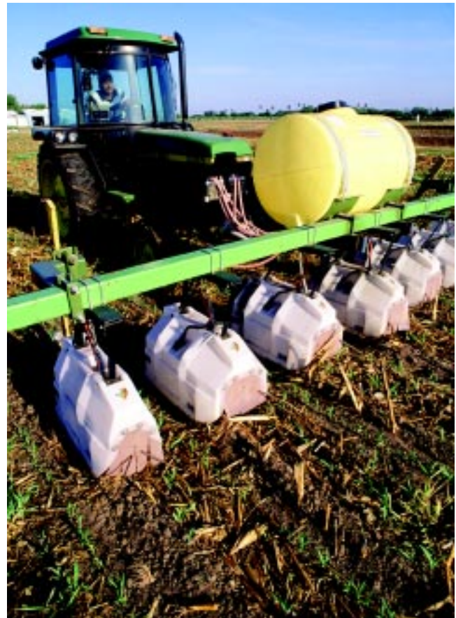
Figure 2.8. Hooded sprayers operated by a field technician direct herbicide just to areas between rows of grain sorghum. Photo by Jack Dykinga, Agricultural Research Service, U.S. Department of Agriculture, Beltsville, Maryland.
