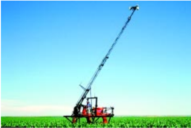
Figure 3.8. Multiband cameras in airplanes or on ground rigs can be used to detect nutrient, water, or disease stress in crop plants. Photo courtesy of P. Westra, Colorado State University.
