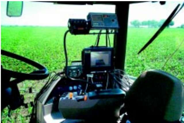
Figure 3.1. To make variable-rate applications, modern farm equipment is equipped increasingly with computers, monitors, global positioning system receivers, and variable-rate controllers. Photo courtesy of P. Westra, Colorado State University.
