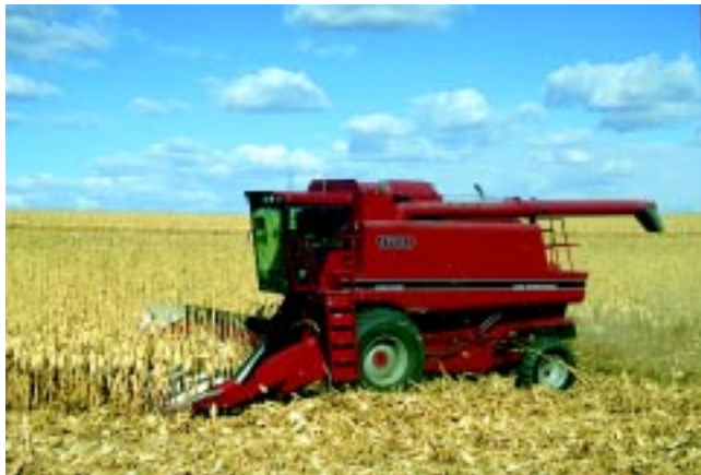
Figure 3.3. Use of a crop harvester equipped with a yield monitor allows generation of a yield map showing yield variability within a field. Photo courtesy of P. Westra, Colorado State University.
