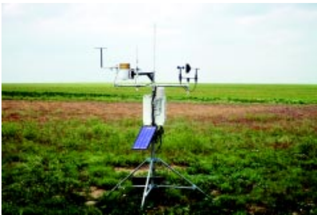
Figure 3.7. Automated weather stations can provide real-time, site-specific weather data that can be used to seed crop-management decision support systems. Photo courtesy of P. Westra, Colorado State University.
