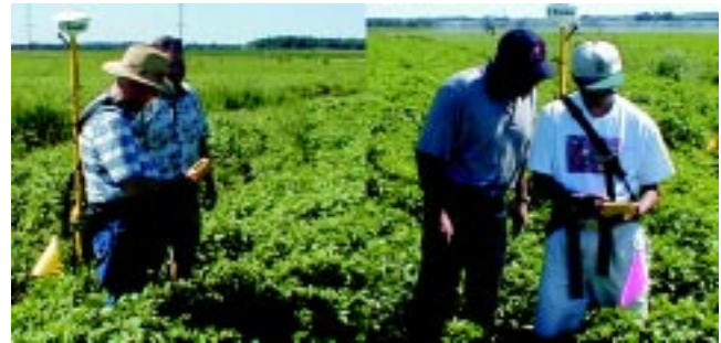
Figure 2.6. Field scouting with "backpack" that allows for georeferencing of information. (Courtesy of W. Stevenson and associates, University of Wisconsin-Madison.)
