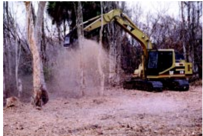
Figure 6.2. Specialized logging equipment is sometimes used to remove invasive tree species. Photo courtesy of F. Laroche, South Florida Water Management District.
