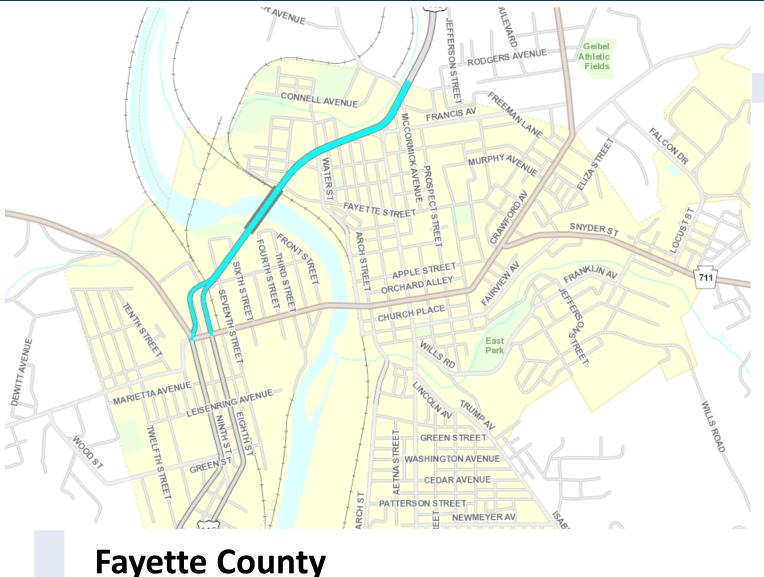
ECMS: 110402 SR 119-SE4 Let Date: 08/10/2023 **Cost Range:** \$1M - \$2M Scope of Work: Full replacement of two (2) existing traffic signals, and upgrades to four (4) existing traffic signals including sidewalk and ADA curb ramp replacement as well as updating the pavement marking and signs.
