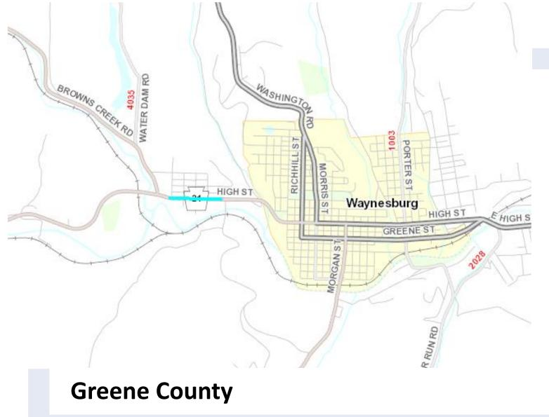
ECMS: 118003 SR 21-0 Let Date: 10/05/2023 **Cost Range:** \$2M - \$3M Scope of Work: This is a safety project on SR 21 in Waynesburg to install a center turn lane in a corridor that is currently a 2-lane, 2-way roadway with many driveways and intersections.
