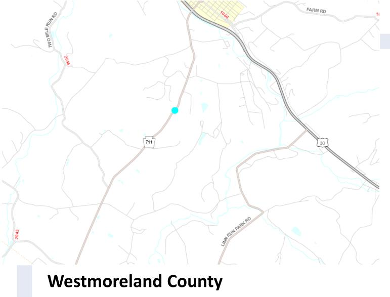
**ECMS:** 31818 SR 711-M10 Let Date: 04/27/2023 **Cost Range:** \$1M - \$2M Scope of Work: Replacement of the existing structure carrying SR 711 over Tributary to Loyalhanna Creek with a 72" reinforced concrete pipe, approximately 200' of stream enclosure with a 72" concrete pipe, three 8' inlet boxes, minor approach work, and other miscellaneous construction.
