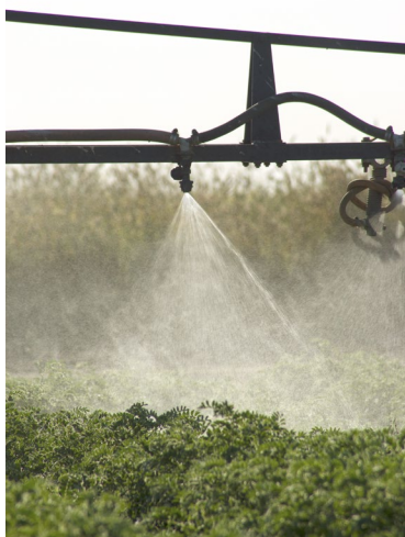
Figure 5-1 Most pesticides are applied with a nozzle type designed to produce a tapered flat-spray pattern, like this one.
