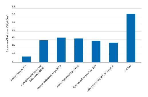
Figure 12. Life cycle emissions of SAF types, compared to jet fuel
