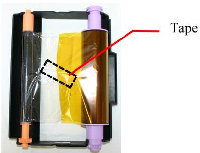
4. Rotate the up-take ribbon several times until the tape is out of sight. Take care that there is no slack in the ribbon.
