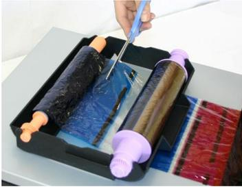
2. Carefully remove any ribbon remaining in the mechanism.
