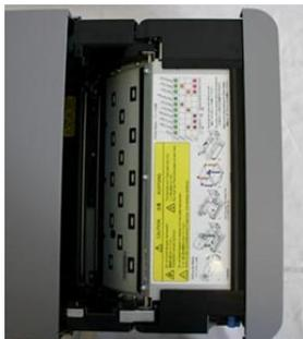
1. Pull any paper remaining in the printer in the direction shown, and cut off any wrinkled or partially printed areas evenly with scissors. Printing over an already printed area will cause the ribbon to stick, and the paper will jam again. When pulling the paper out, pull it slowly. Application of too much force could damage the printer.
