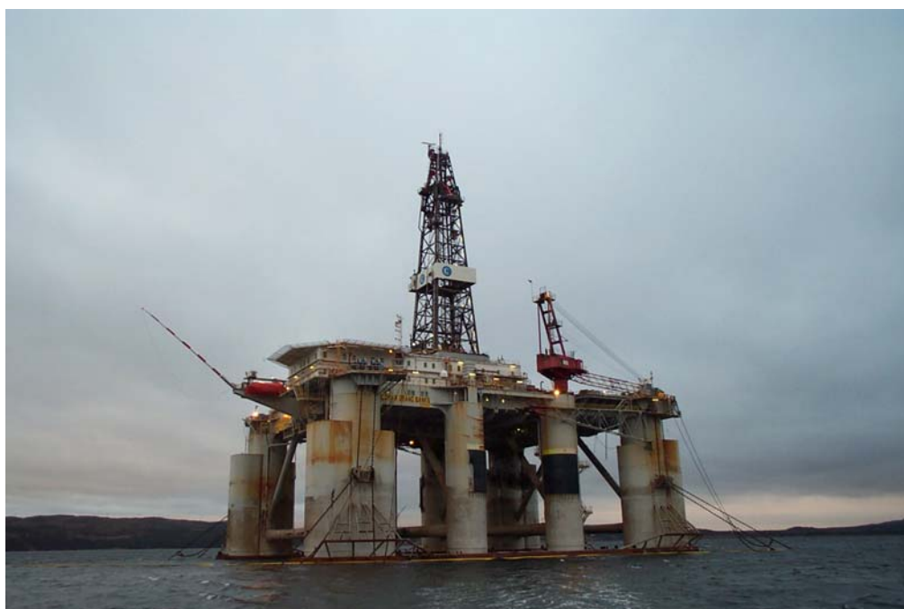
Figure 4.4. Semi-submersible Drill Rig Glomar Grand Banks .
