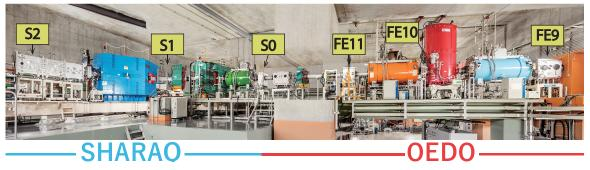
Figure 1. Second half of OEDO beamline and SHARAQ spectrometer.
