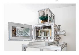
Figure 1. A photograph of CAT-M, which consists of TPC and silicon detectors. The size of active volume is  $310\times280\times200$  mm<sup>3</sup>.
