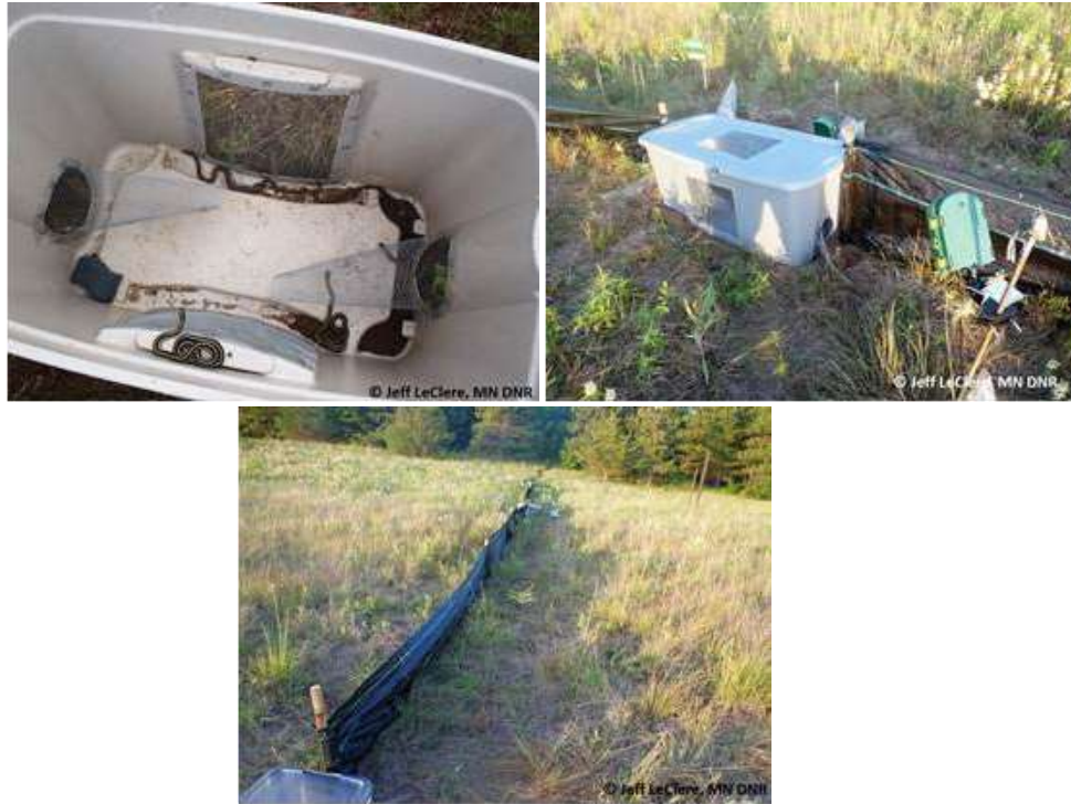
Figure F3 – Photographs of drift fence and box trap setup, the method utilized by the Minnesota Department of Natural Resources (MN DNR). Photos courtesy of Jeff LeClere, MN DNR.
