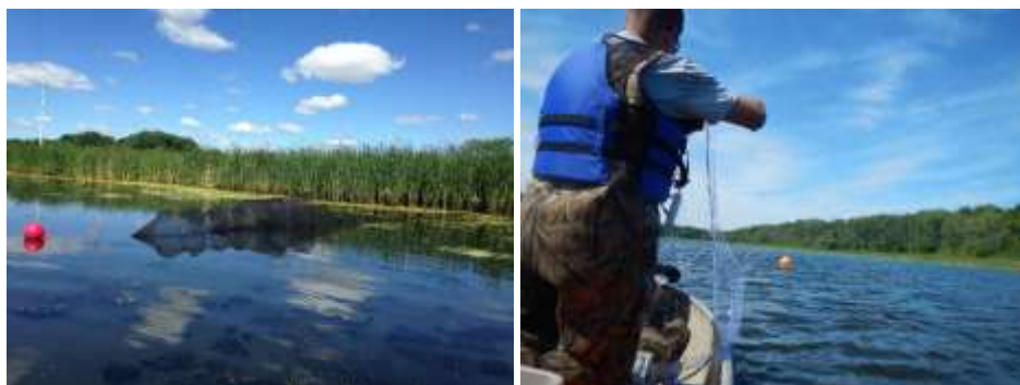
Figure E1. Deployed mini-fyke net (left) and deployment of a gill net (right).
