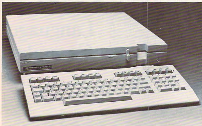
The Commodore 128D computer is functionally identical to the original 128, but sports a new business-style configuration with detached keyboard and a system box with built-in 1571 drive that can support a monitor.
