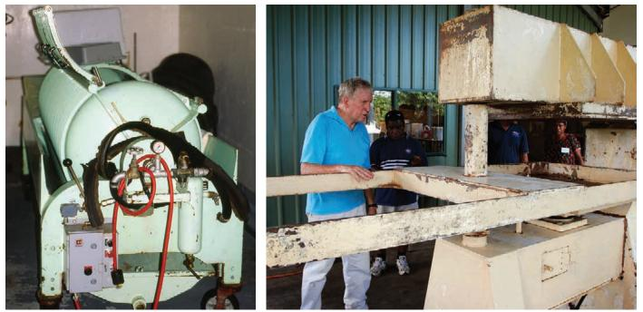
Left: A hydraulic fruit press for making fresh-squeezed noni juice. Ripe fruits are loaded into the press through the top door and juice is pressed from the pulp and bottled immediately. PHOTO: S. NELSON Right: A press for squeezing juice from fermented pulp. Wrapped in special cloth, the pulp is placed into large trays, and the juice is squeezed out by a plate pushed by a hydraulic piston. PHOTO: C. ELEVITCH
