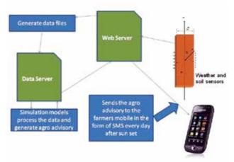
Fig. 94. Work flow diagram of E-Crop
