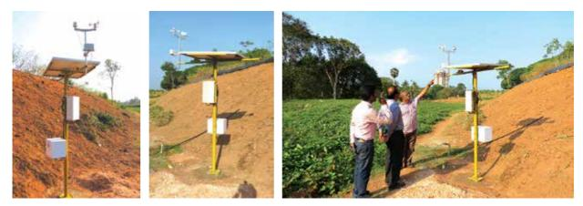
Fig. 92. E-Crop installed in sweet potato field for calibration purpose
