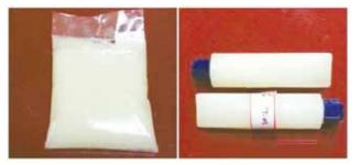
Fig. 83. Binding pastes based on cassava starch
