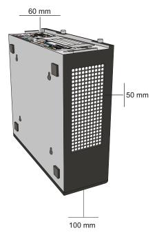
The minimum distances listed in the figure must be maintained; otherwise, a sufficient ventilation of the equipment is not guaranteed.
