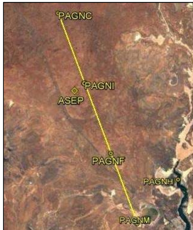
Figure 6.2 RNAV (GNSS) RWY 15 Approach Track and Waypoints and the AESP
