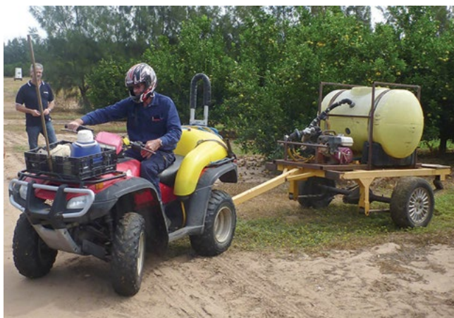
Figure 64. A quad bike towing a Queensland fruit fly spraying rig used by 2PH farms (Emerald). This rig enables higher water volumes to be carried than if using the bike without the tank.
