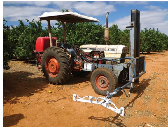
Figure 52. A grower-built trunk band spraying rig.
