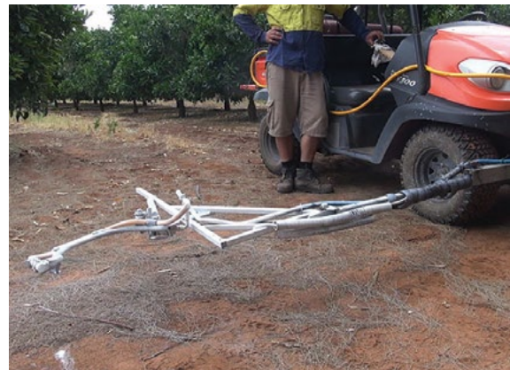
Figure 53. A double-sided trunk band spraying rig that can spray both sides of the tree with one pass.
