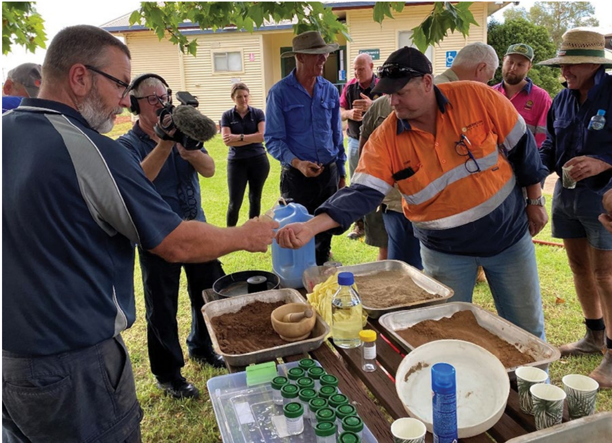
Figure 13. Participants learning how to determine soil texture by rolling moist soil in their hands.
