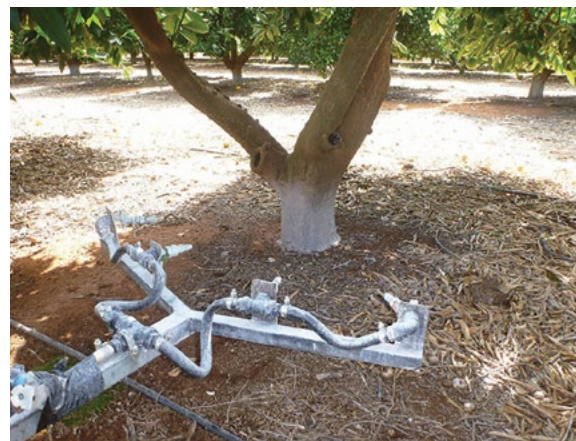
Figure 54. Kaolin clay is added to the insecticide mixture for coverage and overspray inspection.
