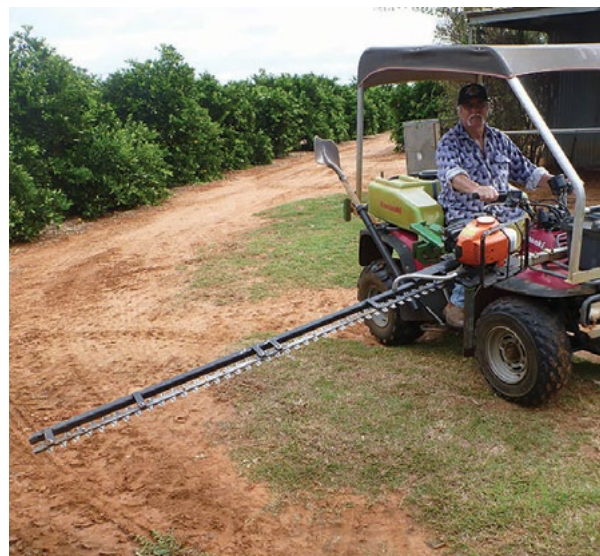
Figure 51. A light gauge skirting bar used to trim the canopy regularly throughout the season.
