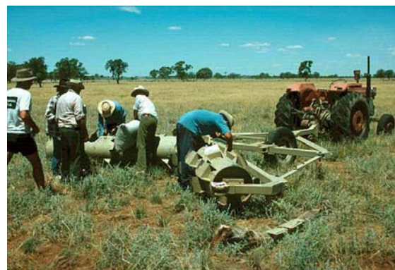
Figure 7. Crocodile seeder showing two drums each with metal feet which cut into the surface as the machine is pulled across the area. The depth of the imprints depends on the offset of the two drums and the softness of the soil surface. [Photo: Tony Grice]
