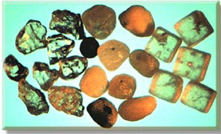
Quartz sand grains compared with cubical crystals of ordinary table salt (NaCl). Left: Angular sand grains from the Algodones Dunes; Middle: Rounded, highly polished sand grains from Sand Mountain, a booming dune; Right: Cubical crystals of ordinary table salt.
