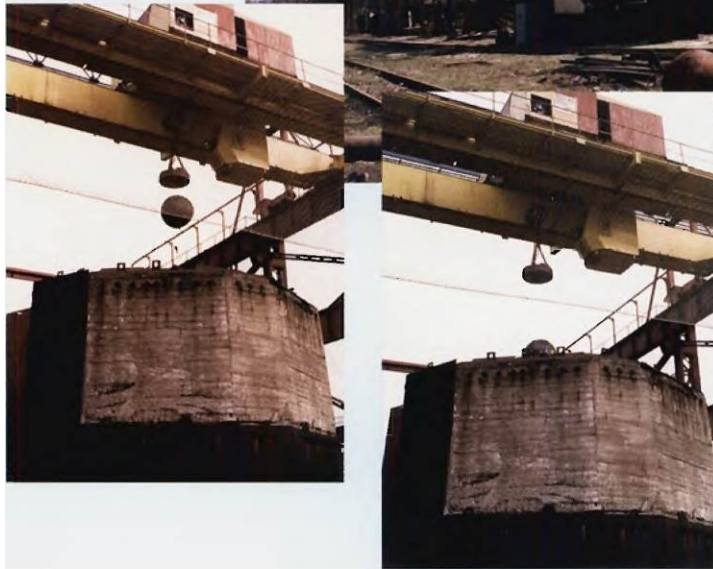
Above and left: Magnetic force releases steel ball from gantry onto TLE in chamber. Below: Crushed relics, the results of smashing by the eight-ton ball.
