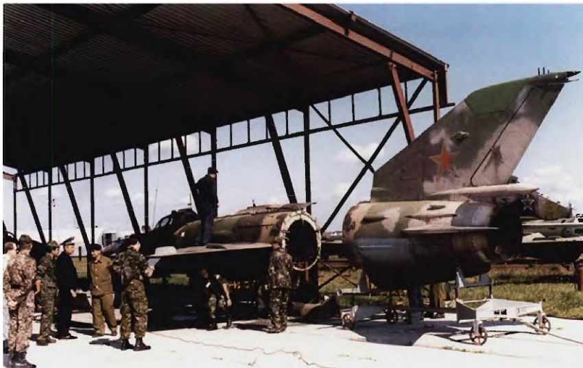
The fuselage was the key component for an aircraft reduction, either by deformation or by severing, as shown on this MiG-21 "Fishbed."
