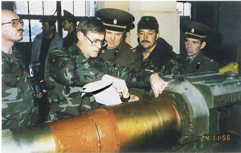
Team Drach checking the length and location of a cut on a gun tube.
