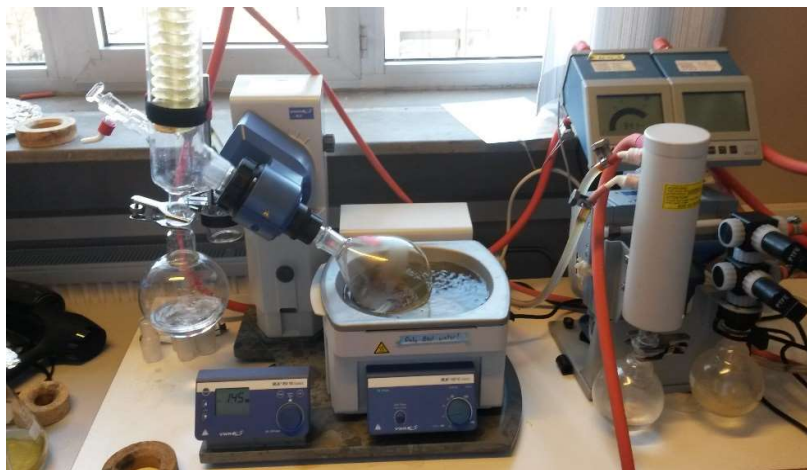
Figure 22. Rotary evaporator for organics solvents with water bath: IKA® RV 10 basic, IKA® HB basic and vacuum pump- Vaccubrand CVC2
