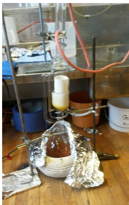
Figure 26. Soxhlet extractor consist of the extraction chamber, the condenser and round bottom boiling flask that heats on heating mantle
