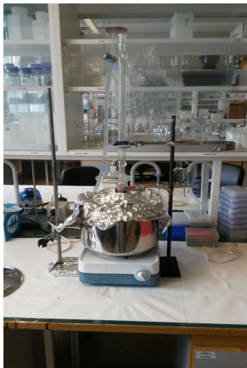
Figure 27. Water extraction: Large bottom flask with mushroom material and purified water in cooking pot as a water bath and reflux condenser
