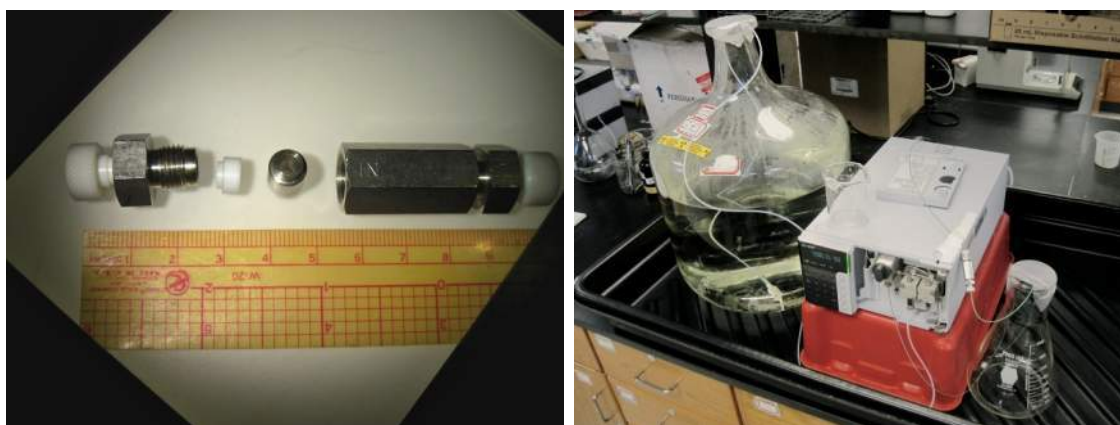
Figure 2-1 Example RSSCT Set-up (Courtesy of Dr. Knappe, NCSU)
