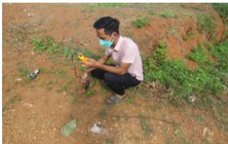
Figure – 46: Measuring vibration at Inn Wine village
