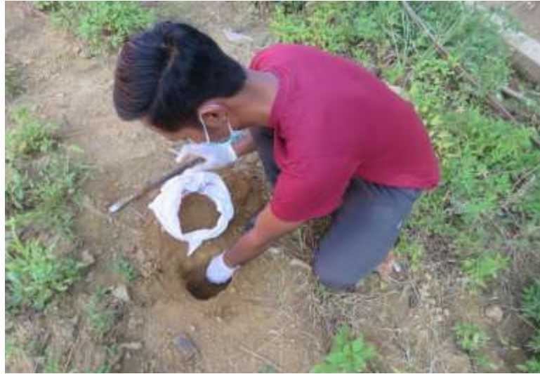
Figure – 38: Taking soil sample from the project site
