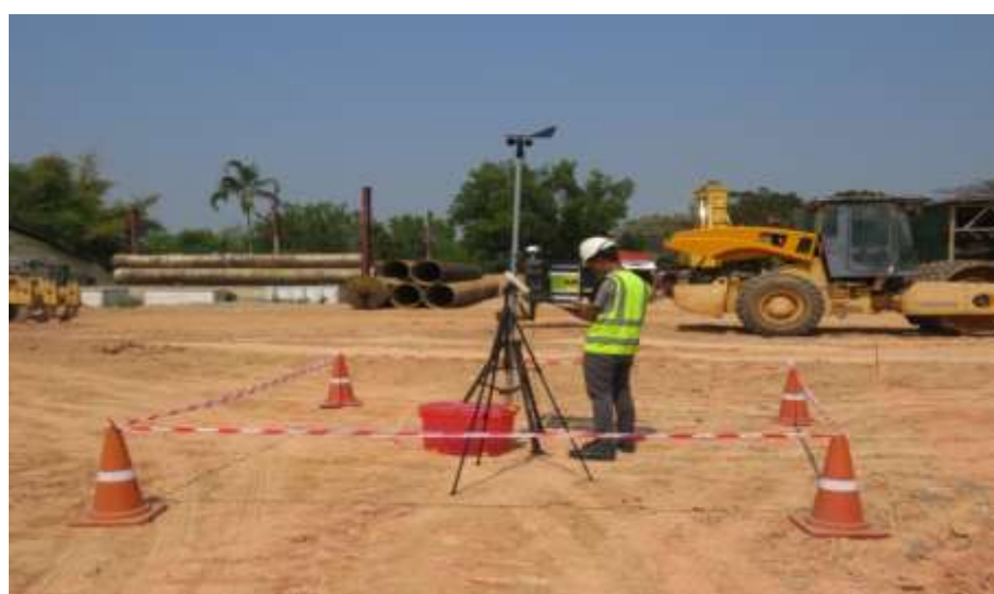
Figure – 50: Measuring ambient air quality
