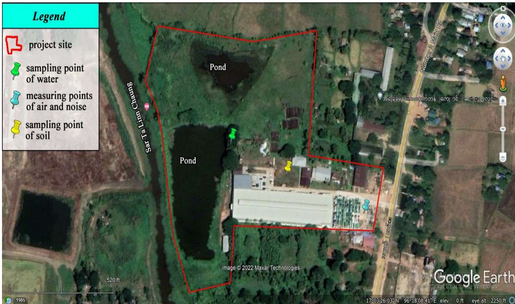
Figure – 52: Satellite image showing spots where air quality and noise level were measured and soil and water samples were taken
