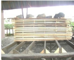
Figure 2: Air seasoning stacks of E. pilularis , E. viminalis and T. dregeana lumbers.
