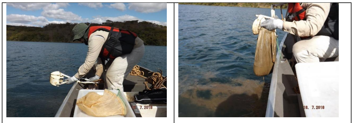
Figure 44 – Benthic communities collection methodology at the Araguari River on July 2018 (collection with Van Veen dredge at left and with nylon net at right)
