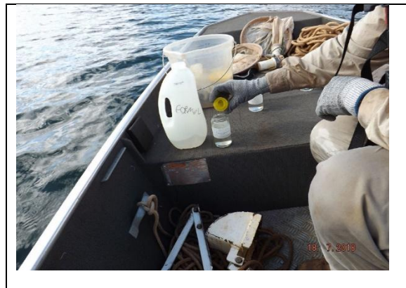
Figure 43 – Planktonic communities collection methodology at the Araguari River on July 2018. Zooplankton fixation with formallin
