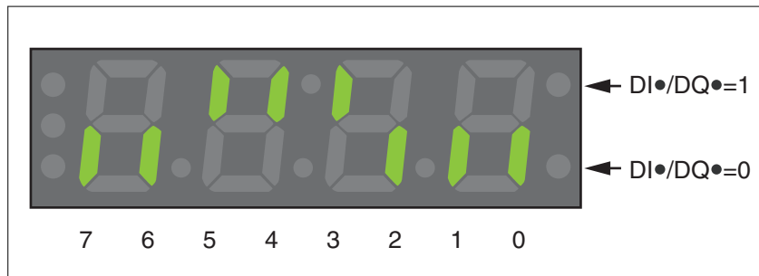
Figure 42: Integrated HMI, displaying the signal state of the digital inputs (DI•) and outputs (DQ•)
