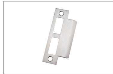
Brass Extended Strike Plate 2 \frac{1}{2} " wide x 4 \frac{7}{8} " high Supplied with Mortise Locks when door thickness is specified as 2" or greater
