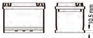
B1 Base holddown 10.5 mm (on long sides)
