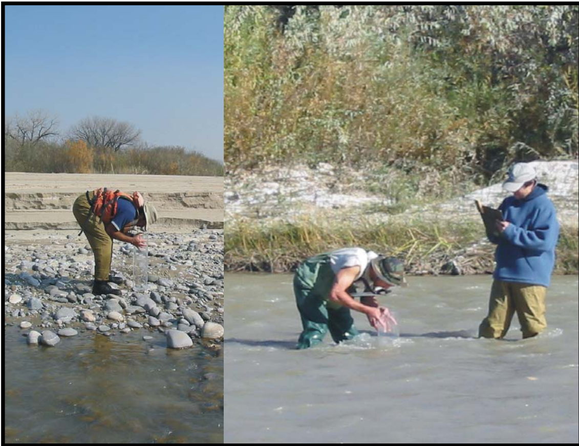
Figure 2.11 - Plexiglas cylinder with a 3 cm grid marked on the base used to record percent surface fines
