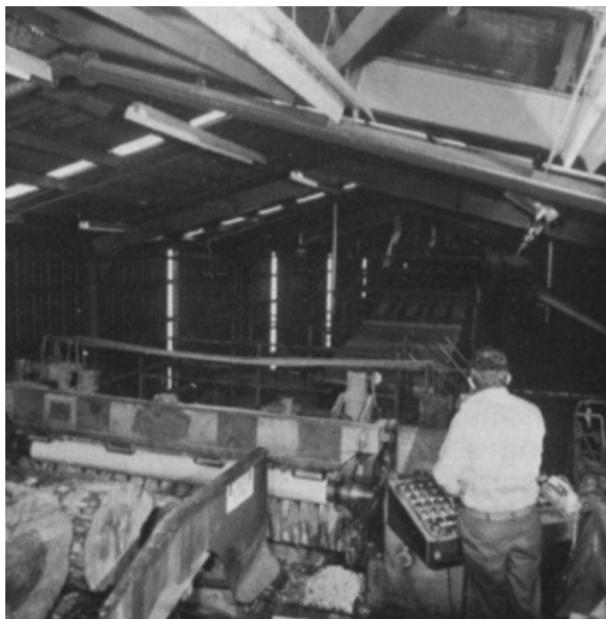
A worker pushes buttons on a console to operate the veneer lathe at the IFP mill. (Forests Branch, Department of the Capital Territory, Forestry in the ACT , c. 1978)
