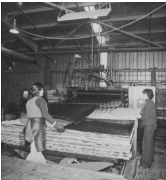
Women handling sheets of veneer glued together during the manufacture of plywood at the IFP mill (Forests Branch, Department of the Capital Territory, Forestry in the ACT , c. 1978).
