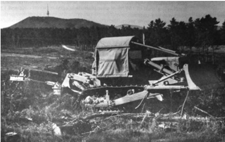
A chopper roller grinds branches of unusable timber and other organic matter into the soil in preparation for planting another crop of pine trees at Stromlo Forest, c. 1985. (Department of Territories, Forestry in the ACT 1984–85 )
