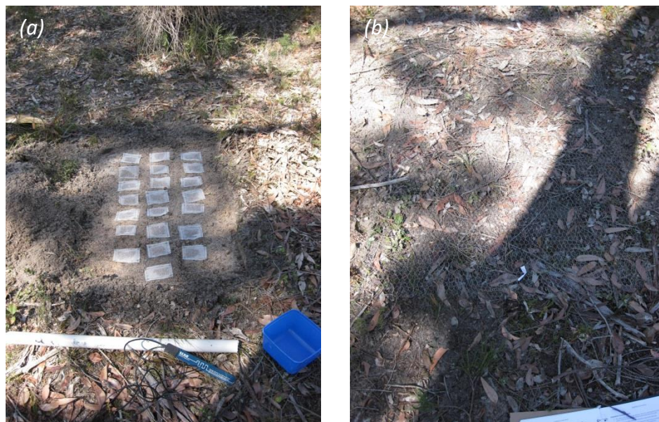
Figure 3.10: Experimental layout of burial trial. (a) Positioning of bags in one replicate. (b) the same replicate once bags were buried, leaf litter returned and wire netting placed over the area.
