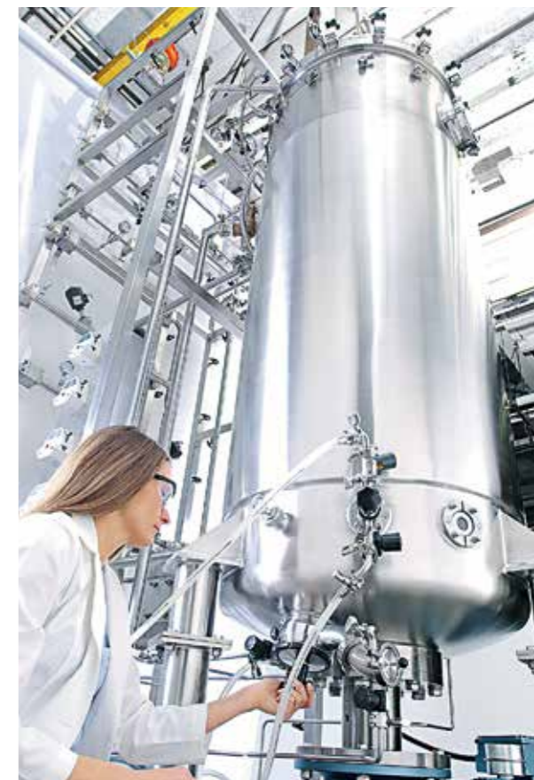
BioFlo Pro fermentors offer working volumes of up to 1,200 L.
