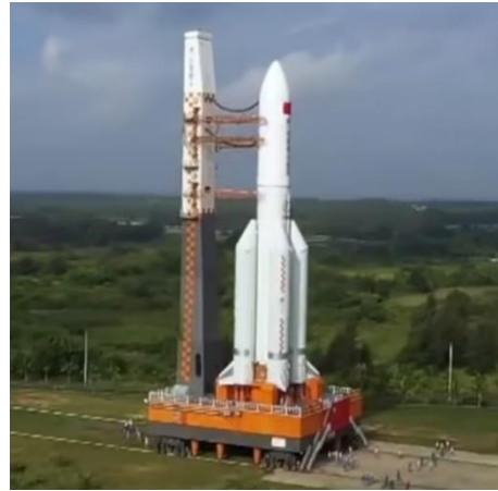
With the maiden flight of Long March 5B, China successfully tested its most powerful rocket yet, designed to lift up to 22 tons to LEO. Even more capable launchers are in development (Credit: CGTN / Youtube)
