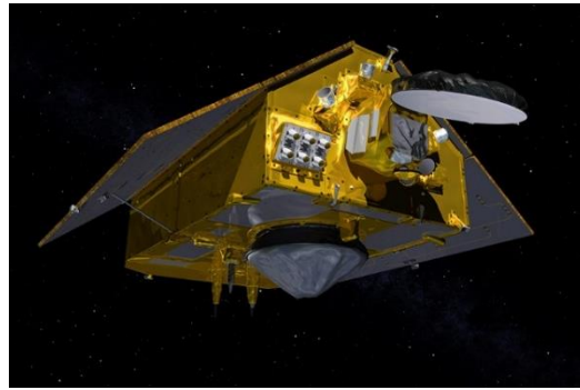
Sentinel-6 Michael Freilich satellite, launched in November, will conduct its oceans-observing mission from an orbit with a nominal altitude of 1336 km and 66° inclination (Credit: EUMETSAT)
