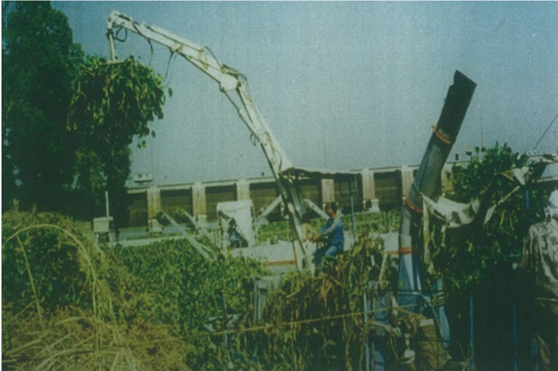
Figure 7. Harvester used for water hyacinth
