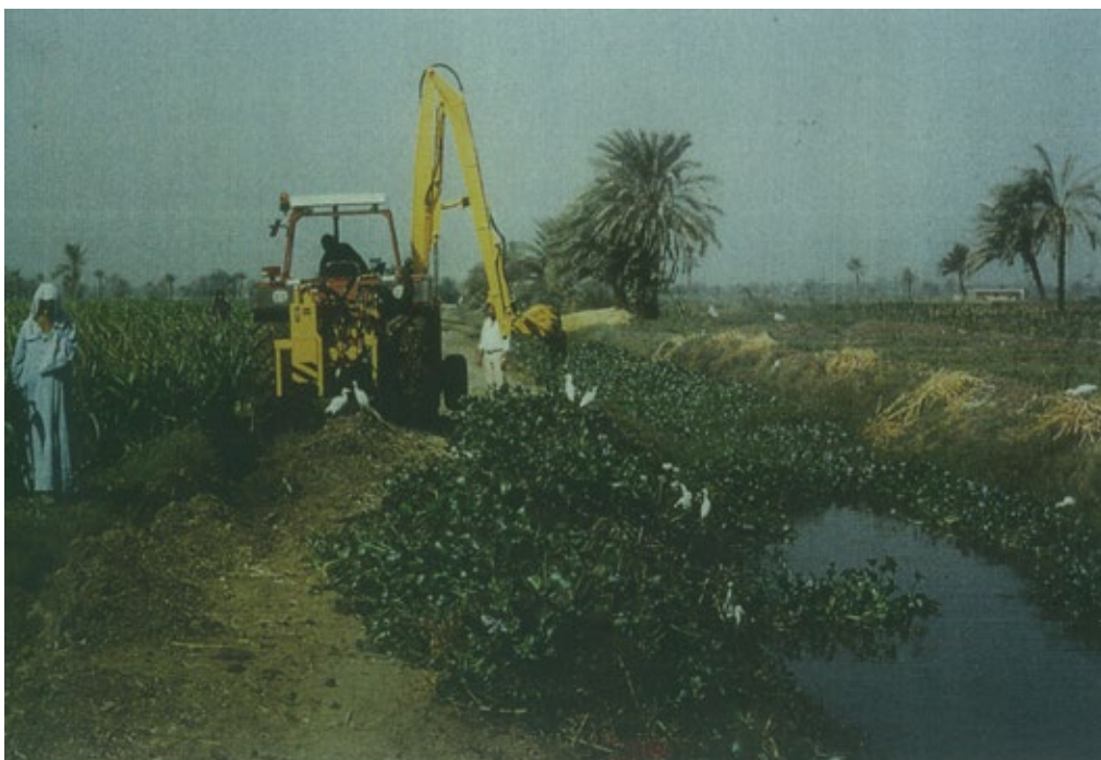
Figure 9b. Weed mowing bucket in action
