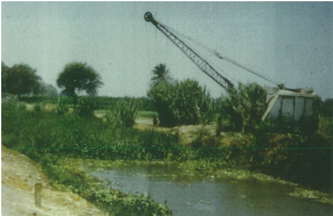
Figure 8. Dragline used for water hyacinth control
