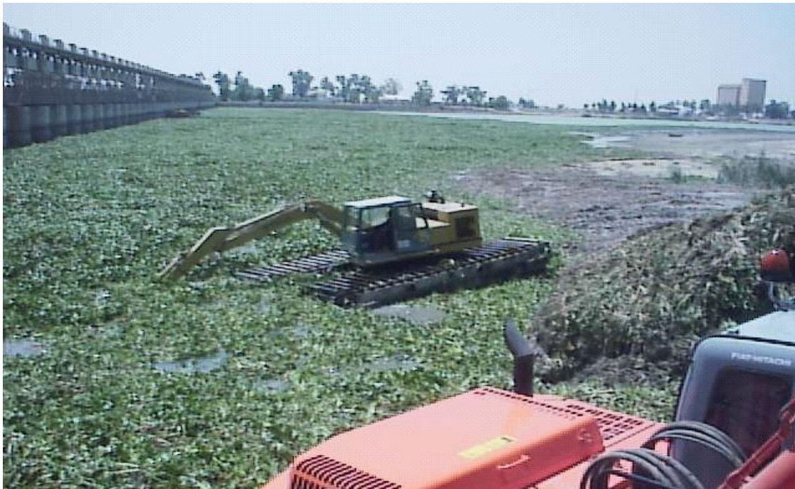
Figure 6a. Harvester used for mechanical control of water hyacinth in Iraq
