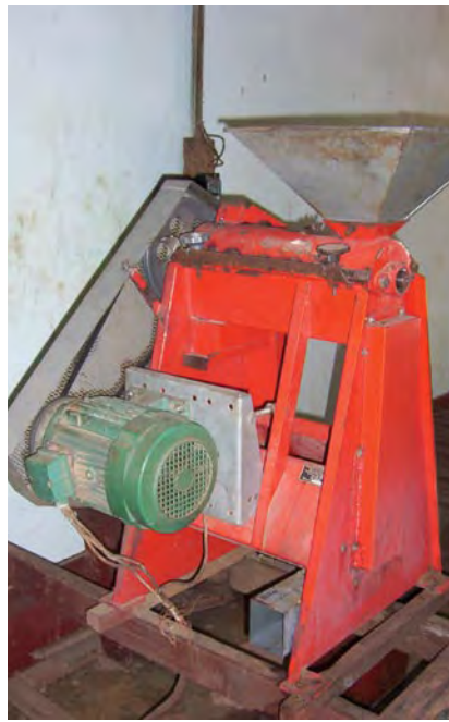
Figure 36. Hulling machine (above) and beans with parchment removed after hulling (right)
