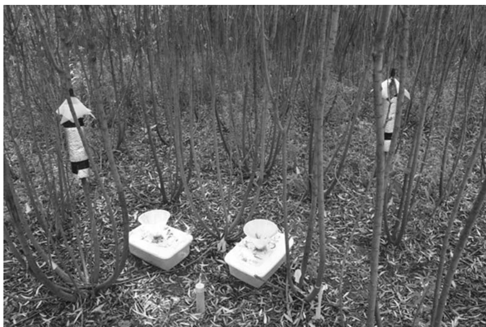
Fig. 6.31. Three-year-old willow trial on the Solvay wastebeds where sapflow, throughfall, soil moisture and various plant characteristics are being measured as part of the effort to develop an alternative vegetative cover for the wastebeds. Photo courtesy of T. Volk.
