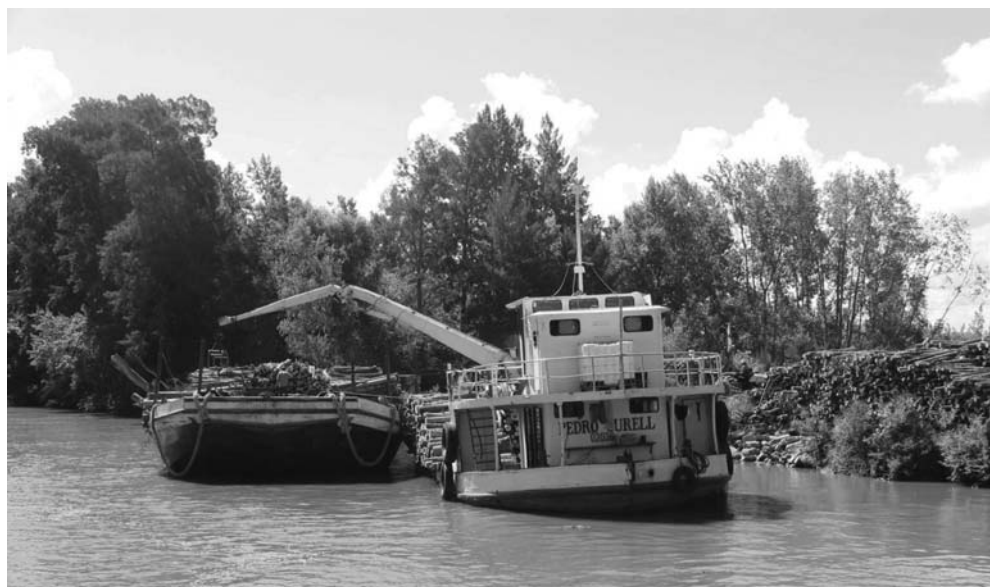
Fig. 5.21. Where plantations are located close to a major river system, barges may be used to transport chips or logs to the mill. Most transport is by barge in the Paraná delta of Argentina; here poplar logs are being loaded on to a barge. Photo courtesy of J. Stanturf.
