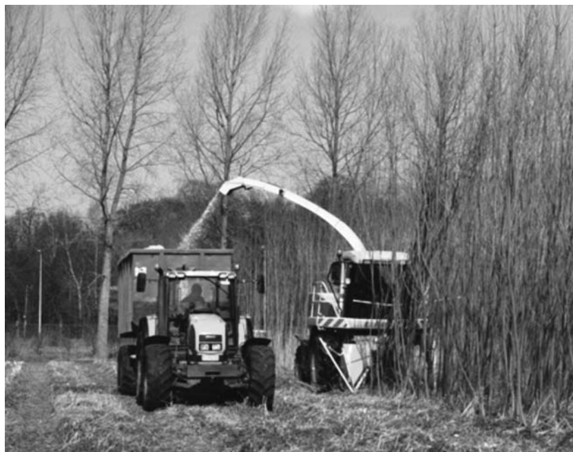
Fig. 5.23. Silage or maize harvesters with specially designed cutting heads cut, chip and blow willow material into wagons in one continuous operation. Direct-chip harvesting is preferred for bioenergy production because chip quality is better if fresh material is chipped, as opposed to dried whips or bundles. Shown here is a Claas Jaguar direct-chip harvester. Photo courtesy of Claas Group.
