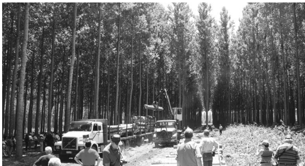
Fig. 5.20. Poplar logs are loaded on to trailers by a crane and transported to the mill. Felling, delimiting and bucking are done manually, by chainsaw crews. Photo courtesy of J. Stanturf.
