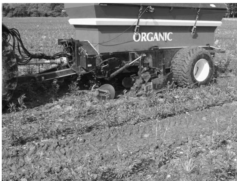
Fig. 6.28. Biosolids injection into freshly coppiced SRC willow. Photo courtesy of Rural Generation Ltd.
