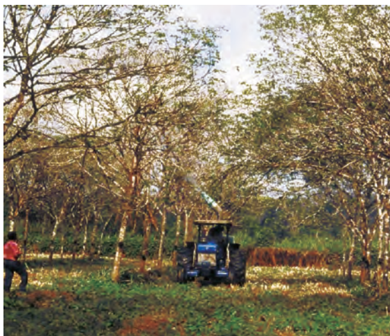
Figure 12. Spraying of fungicides using a tractor-mounted mistblower
