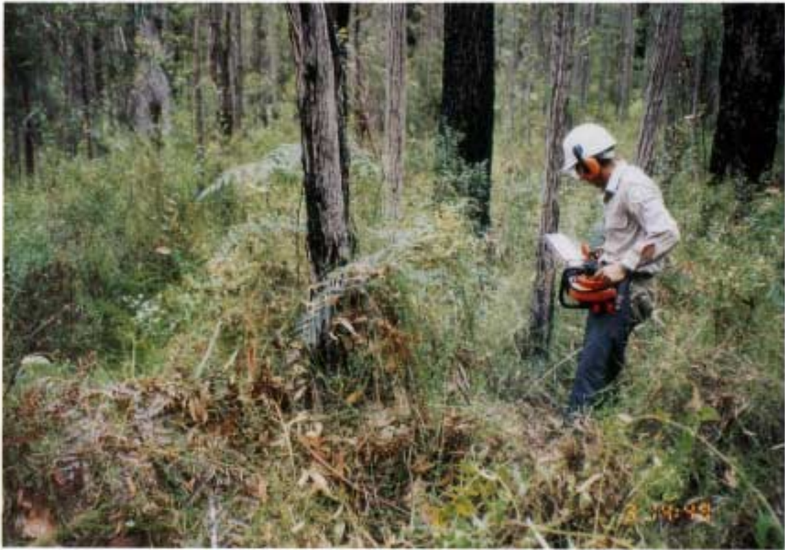
Photograph 3 Destructive sampling of elevated fuels using mechanical hedge trimmers. The wiregrass fuels being sampled are 24 years old, with a fuel load that comprises 8.1 t/ha of elevated fuel, and 13.7 t/ha of surface litter. The average height of the elevated fuel is 1.4m and the cover is 70%.
