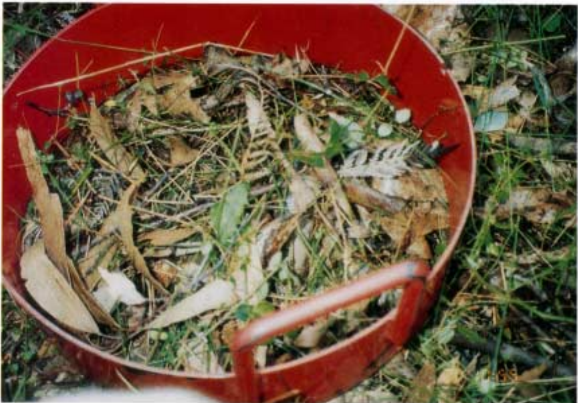
Photograph 4. Sampling frame (0.1m 2 ) used for the destructive sampling of surface litter fuels. The surface litter fuels being sampled are four years old, with a fuel load of 5.5 t/ha and a litter depth of 22 mm.
