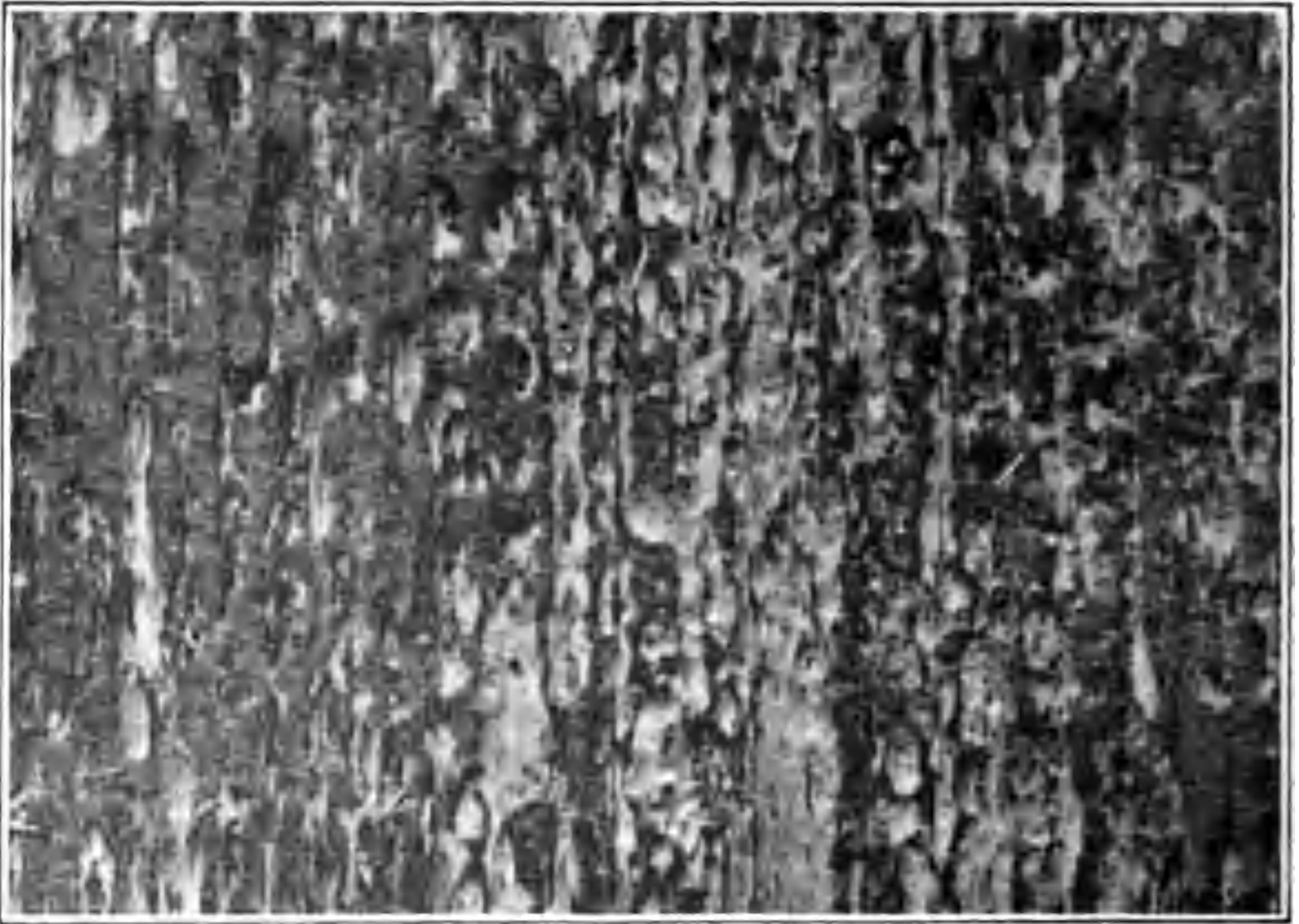
FIG. 65. — Advanced stage of pecky wood-rot in longitudinal section.
